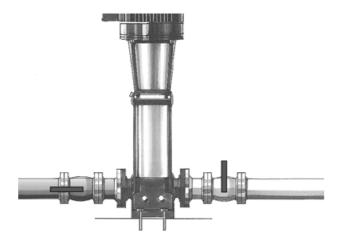
1. Close the isolating valve on the pressure side of the pump and open the isolating valve on the suction side.
