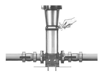
7. Close the vent valve when a steady stream of liquid runs out of it. Open the discharge isolating valve fully.
