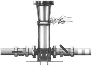
6. Continue to vent the pump. At the same time, open the discharge isolating valve a little more.
