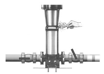
5. Vent the pump by means of the vent valve in the pump head. At the same time, open the discharge isolating valve a little.
