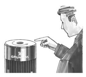
3. See the correct direction of rotation of the pump on the motor fan cover.
