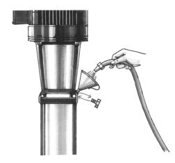
2. Remove the priming plug from the pump head. Pump is vented through filling out of the receiver. If necessary slowly fill the pump with liquid. Replace the priming plug and tighten securely.
