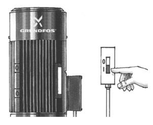
Start the pump and check the direction of rotation
