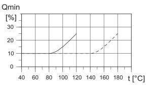
Because of the risk of overheating, the pump should not be used at flows below the minimum flow rate.
